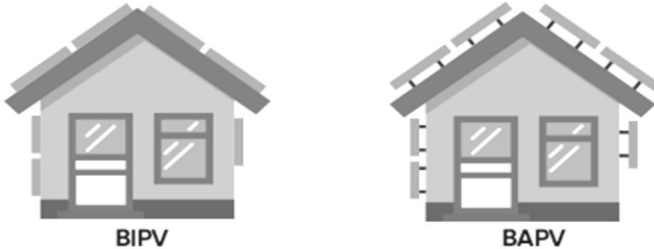
(Fig. 7) , Classification Concept of (PV) application in Building, as (BAPV & BIPV) [Ref. [19], Adapted by author].
