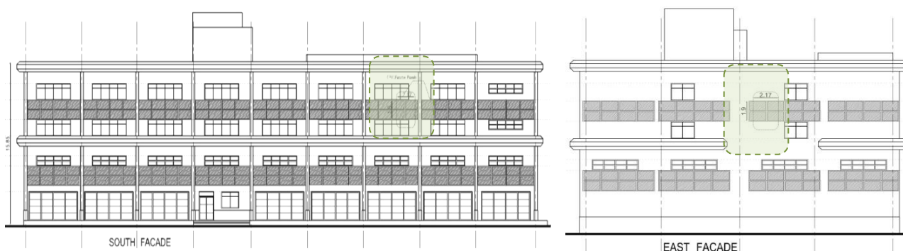
(Fig. 10 ( b) – “Case-Study”: (PV) Panels module application on (South & East) Façades , [Drawings by Author]
